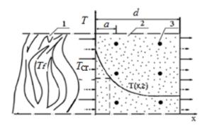
Fig. 2 – Typical thermo-technical scheme: 1-fire, 2-concrete, 3-reinforcement, d-member width, *a*-concrete cover depth,  $T_{cr}$ -critical temp.,  $T_f$  -fire temp.,  $T_{x,r}$ -temp. profile [2]
