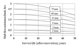
Fig. 4 – Fire resistance limit of reinforced concrete slabs of pre-cast residential buildings based on service condition and service life  $(l_y A_x \ge 1.5)$
