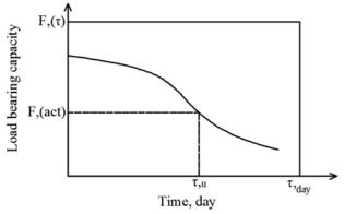
Fig. 1 – Typical scheme for the assessment of fire resistance by strength reduction criterion at elevated temperature [2]
